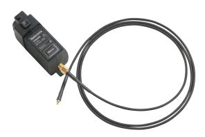
The TPR1000 and TPR4000 probes provide a low noise, large offset range solution for measurement of ripple on DC power rails ranging from –60 to +60 VDC. Tektronix's power rail probes offer industry leading low noise and high offset range required to measure AC ripple between 200  $\mu V_{p\text{-}p}$  and 800 mV $_{p\text{-}p}$  at up to 4 GHz.
